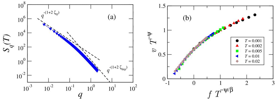
**Fig. 6.** (a) Structure factor  $S_q$  at a finite temperature  $T = 0.02$ , showing two regimes with different roughness exponents,  $\zeta_{FF}$  and  $\zeta_{dep}$ , above and below the crossover length scale  $\ell_{av}$ , respectively. (b) Velocity–force scaling function in the thermal rounding region. The disorder intensity is kept fixed and the velocity for different temperatures collapses in a single function. Figures are adapted from [50]. Color available online.
